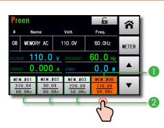
To create a complex sequence on the HMI is no longer a difficult task for AFV-P series. The 5 inches touch screen provides users a clear display and an easy set up. AFV-P series can display 4 shortcuts of Memory Sets, and the voltage and frequency setting of each Memory Sets can be clearly read. The user can quickly switch the output by selecting the shortcuts.
