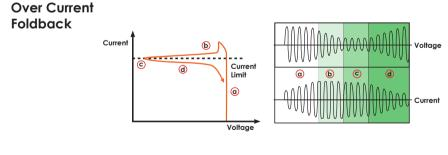
When it comes to over current, AFV-P series offers more than just shutdown protection. Over current foldback enables AFV-P series to maintain the output current at the rated current and correspondingly decrease the output voltage as the load impedance increases. It is an extended protection or an alternative to provide constant current for EUT.
