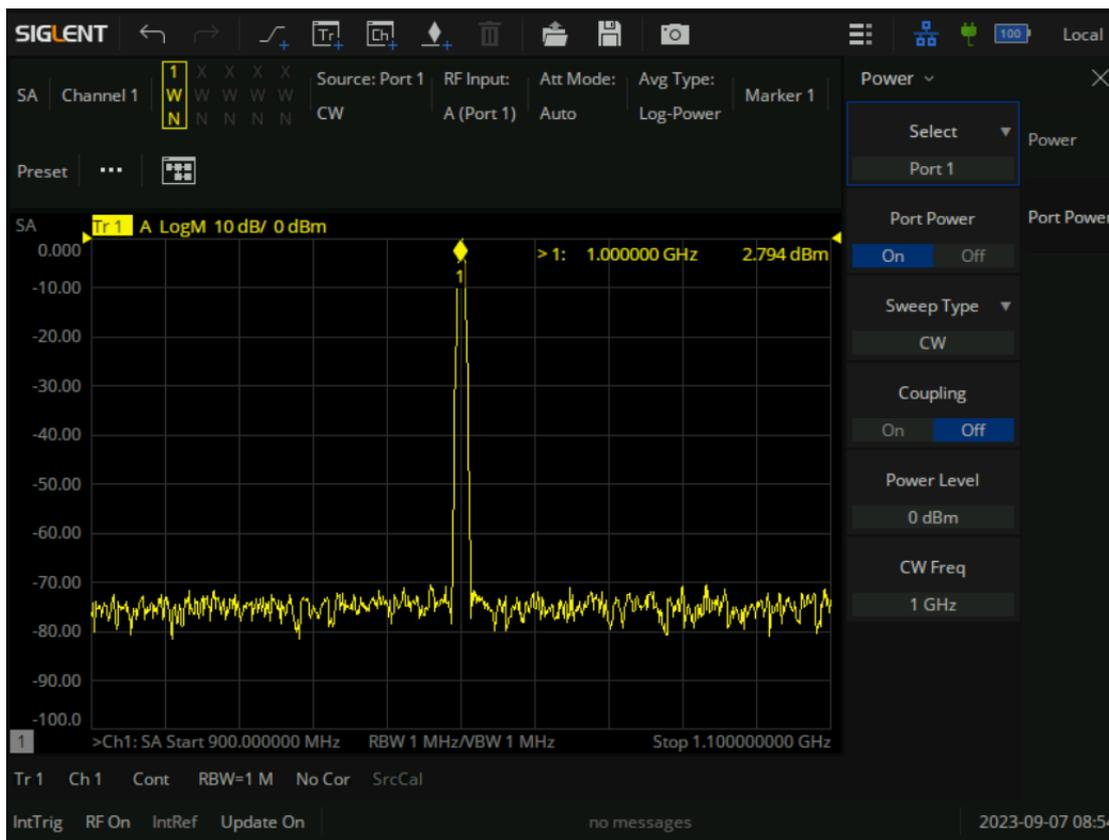
Figure 9-8 Press the [Power] key to enter the source's setting menu
