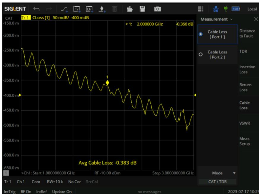
Figure 11-8 Cable loss measurement interface
