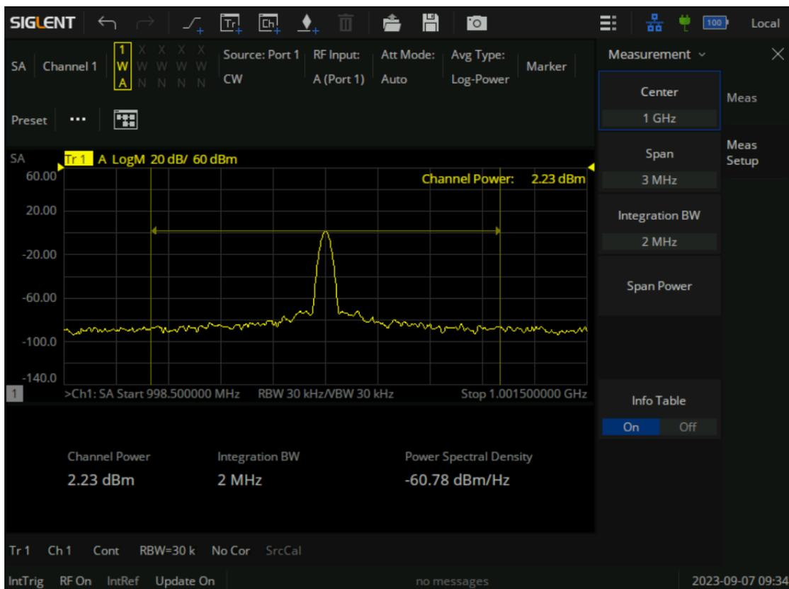
Figure 9-12 Channel Power measure
