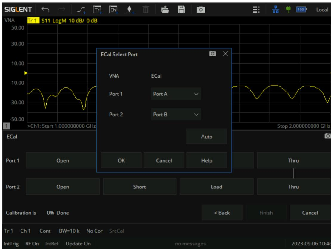
Figure 6-42 Manual port setting
