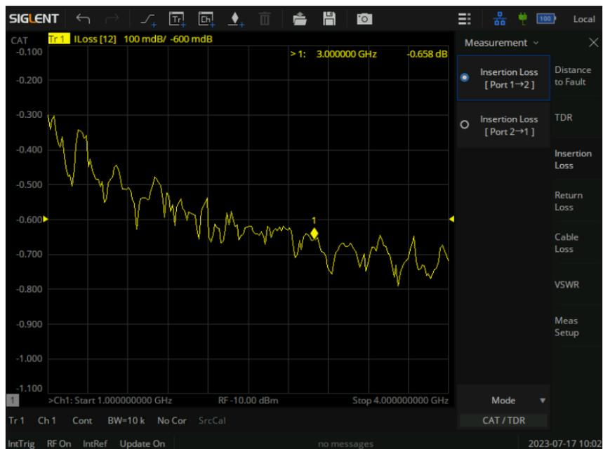
Figure 11-6 Insertion loss measurement interface
