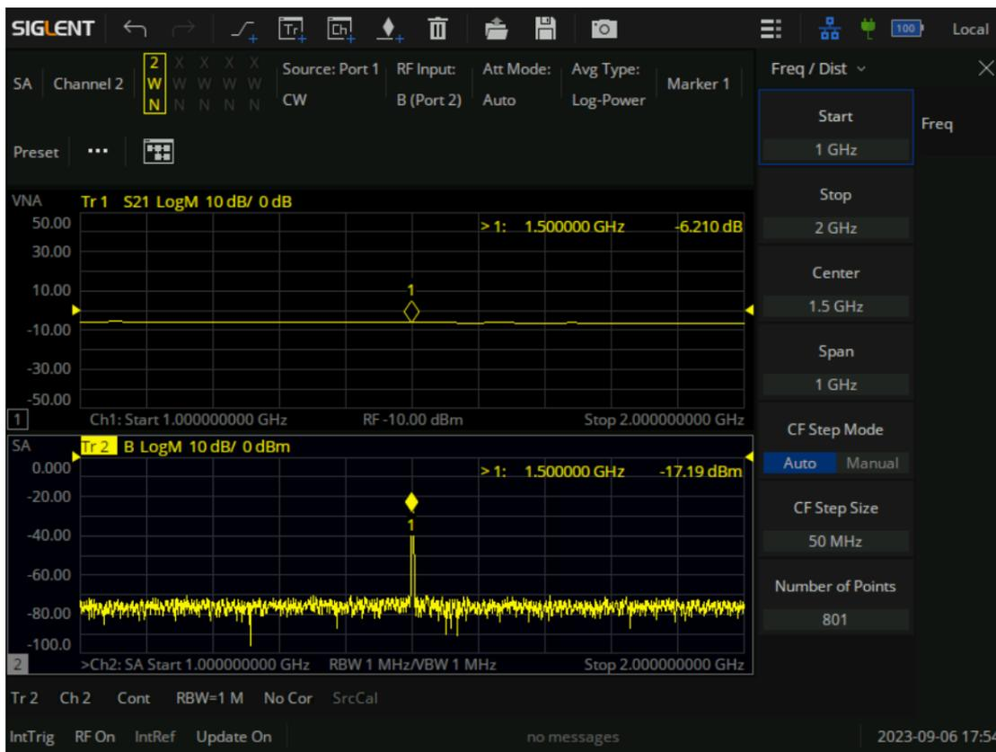
Figure 9-3 [Freq] key to set SA frequency parameters
