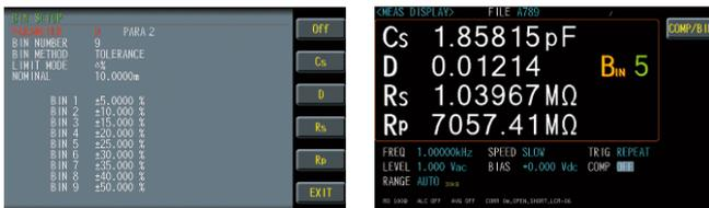
BIN settings for one specific parameter of the selected measurement parameters provide up to 9 BIN positions. Set the judgment basis for individual classifications according to the desired BIN methods (EQUAL/SEQUENTIAL/TOLERANCE/RANDOM) and limit value mode (VALUE/delta/delta%). The result of this sorting can be obtained through the Handler interface. If directly connected to an external device such as a sorter, an immediate sorting can be performed.
