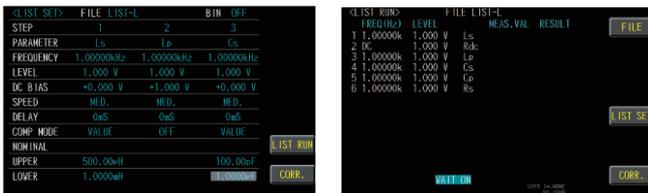
The 15-point LIST measurement mode provides measurement values at a specific frequency or voltage of the DUT, and each set point can set independent comparison and judgement. When the trigger mode is set to "AUTO", the display "WAIT ON" will appear on the measurement screen and LCR-8200 will detect the contact status of the fixture. When the DUT is connected, the test will start automatically.
