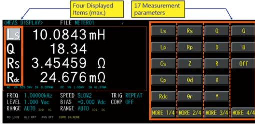
LCR-8200 allows users to select and arrange measurement parameters. Users can select at least one parameter to maximum four parameters from the 17 measurement parameters according to the measurement requirements and the presentation order can also be arranged in a desired manner. The set parameters can be stored in internal/external memory groups for subsequent recalls.
