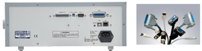
Provides a variety of standard PC connection interfaces such as RS-232C, USB device, LAN, and GPIB industrial control interface to remotely control settings or read measurement results and other related information so as to substantially increase work efficiency without having to pay for additional interface procurement costs. In addition, LCR-8200 also provides Handler interface for PLC external control or for the collocation of measurement integration of sorters.
